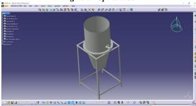
Fig no: 6 Frustum shaped gravity assisted water purifier with spiral tube filter
